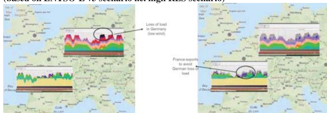
Figure 5 – illustration of cooperation in variability of RES generation across Europe (based on ENTSO-E v3 scenario i.e. high RES scenario)
