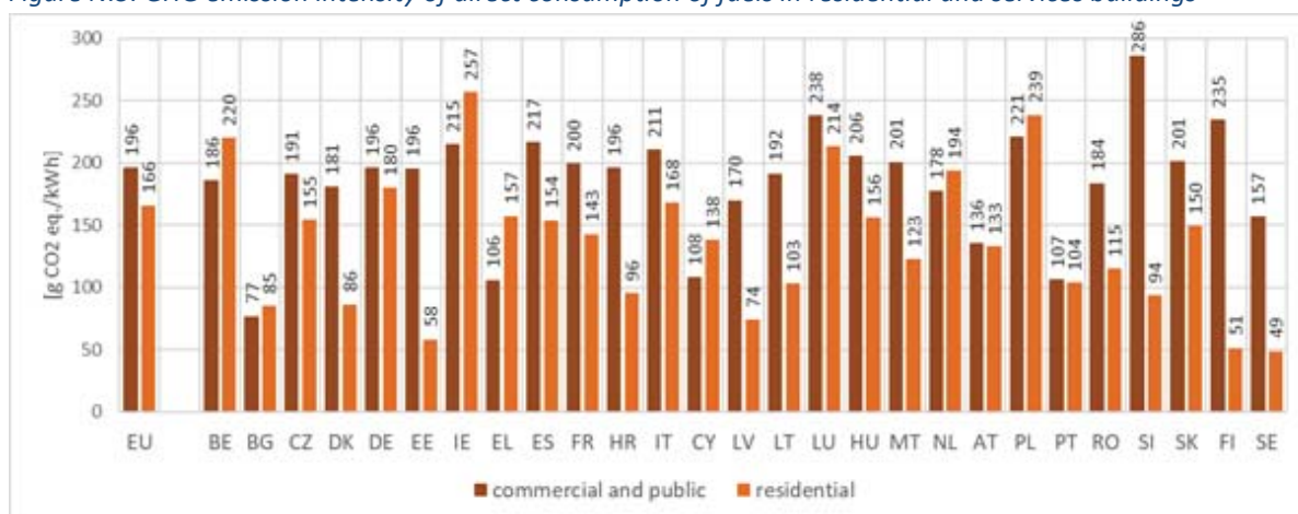
Figure N.5: GHG emission intensity of direct consumption of fuels in residential and services buildings 21
